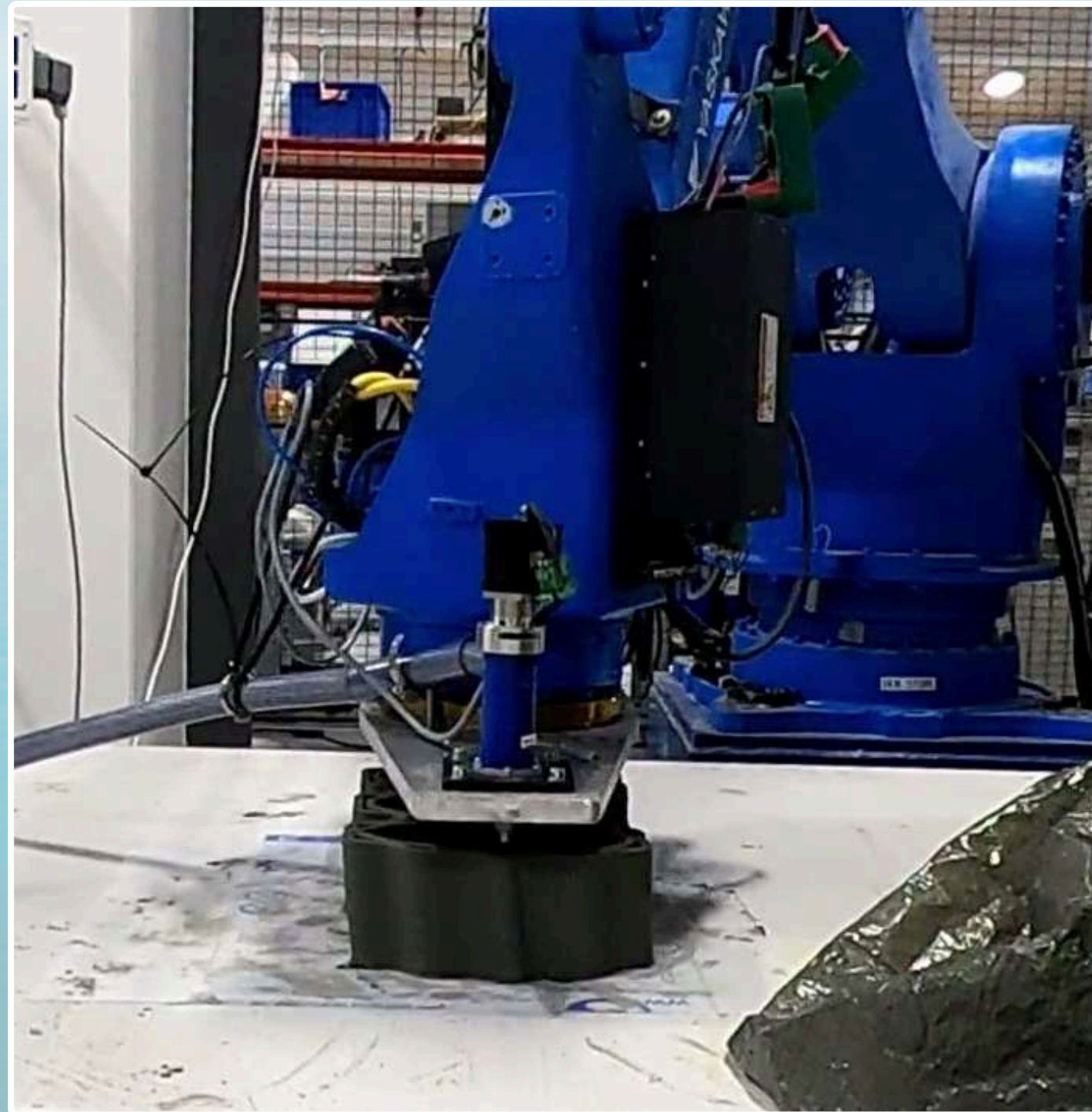
Clay 3D printing utilizing a robotic arm
